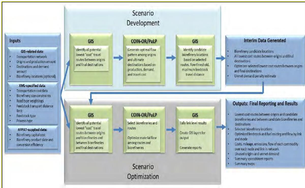
**Fig. 3.2. Analytical Data Flow Schematic for FTOT (Adapted from Lewis et al., 2015)**
