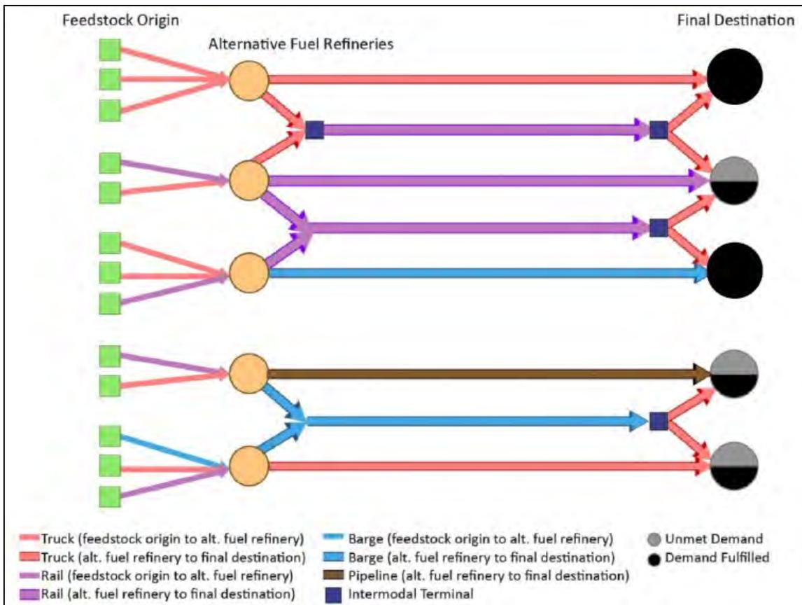
**Fig. 3.3. Levels and Modal Structure of Optimized Network (Adapted from Lewis et al., 2015)**
