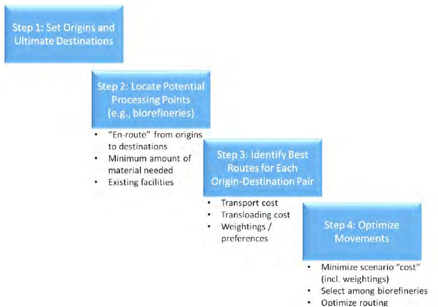
**Fig. 3.1. Analytical Approach of Fuel Transportation Optimization Tool
